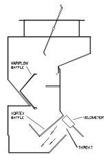
Hold the instrument perpendicular to the VORTEX BAFFLE and parallel to the throat (inlet slot) of the ventilator. Velometer should not exceed three inches in diameter.
