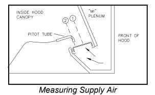
Calculate the average velocity along the length of the perforated discharge and refer to chart No. 2 for corresponding CFM/ft (I/s/m). If the supply air is too high adjust the opposed blade dampers on top of the filter hood at the supply air inlets just above the supply fire dampers. Multiple
