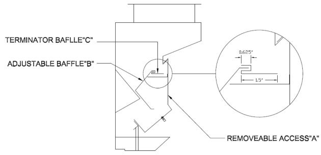
The TBDD Terminator baffle is available in various lengths to suit adverse site conditions. This will provide additional exhaust air over heavy appliances that are being effected by the surrounding environment.
