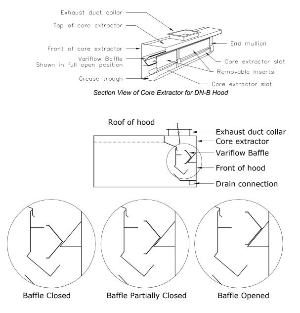
Section View of DN Extractor with Detail of Vari-flow Baffle
