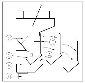
The SPRING AIR SYSTEMS type "D" extractor is a high efficiency dry extractor. The type "D" extractor removes grease, dirt and lint through centrifugal force. Remove the front access door and wipe the interior with a damp cloth to manually wash the extractor chamber.
