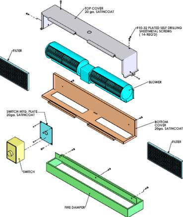
Exploded View of MJ Blower assembly Figure 21
