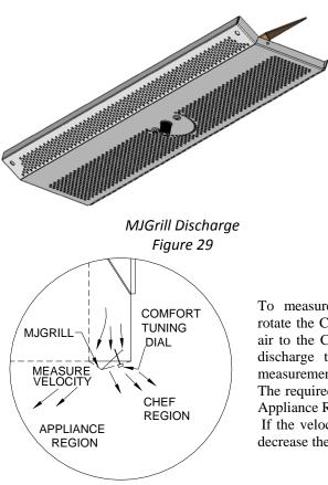
The Appliance Region and Chef Region discharge is called a MJGrill. The MJGrill is manufactured as a single component shown on the left in Figure 29. The MJGrill includes the Appliance Region discharge, Chef Region discharge, and a adjustable Comfort Tuning Dial. The Comfort Tuning Dial proportions the amount of fresh air to the Chef Region.
