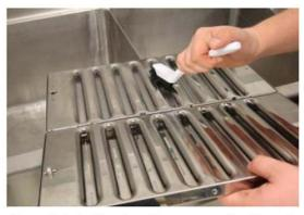
Cascade's locking handles open up the hinged desian. allowing wide-open cleaning access. Cascade shown in the Open Position Figure 18
