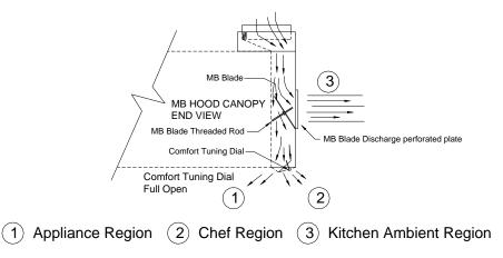
Dynaflow MB Three Regions Figure 28 Each of the three regions must be measured to ensure proper hood operation. The Appliance Region, the Chef Region and the Kitchen Ambient Region as shown in the schematic Figure 28
