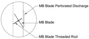
MB Blade Discharge perforated plate There are two sizes of MB Blade Discharge Grills.
