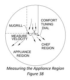
The Appliance Region and Chef Region discharge is called the MJGrill. The MJGrill is manufactured as a single component shown on the left in Figure 28. The MJGrill includes the Appliance Region discharge, Chef Region discharge, and a adjustable Comfort Tuning Dial. The Comfort Tuning Dial proportions the amount of air to the Chef Region.
