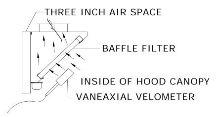
Measuring baffle filter exhaust Air with Vanaxial velometer Figure 24
