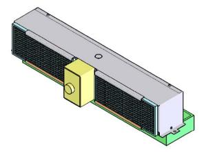
The MJ blower assembly is located on top of the MJ plenum. Each hood has one or more MJ Blower assemblies. To adjust the air flow of the MJ blower rotate the rheostat in the middle of the MJ blower assembly. Rotating the knob clockwise increases the air flow and rotating the knob counter clockwise decreases the amount of air into the plenum. Adjust the know until the correct velocity is measured one the MJ Grill appliance discharge.
