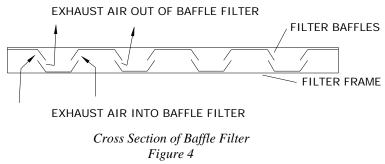
Always ensure that the grease filters are installed with the weeping holes down toward the grease trough. The exhaust air travels into the exhaust plenum, fire damper, exhaust duct collar and then into the exhaust ductwork.
