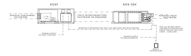
Remote wiring of KES Enviro units with Dry Hood Figure 12
