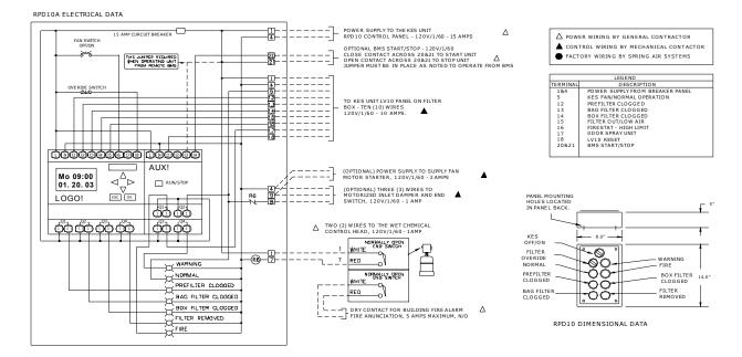
RPD10 Wiring Schematic Figure 9
