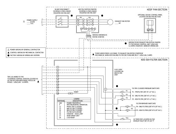
Typical indoor KES, motor starter, LV10 J-Box with odor spray wiring schematic Figure 14
