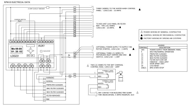
*RPW10 Wiring Schematic* Figure 5
