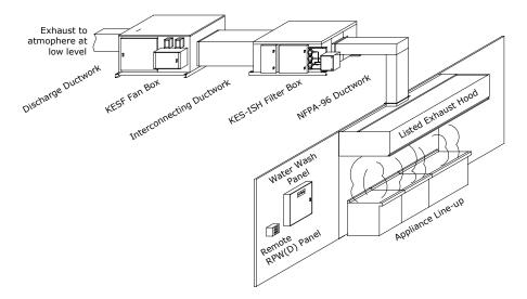
into the exhaust ductwork. The exhaust ducting is connected from the hood to the inlet of the KES Enviro unit. This exhaust ductwork must be supplied and installed in accordance with the NFPA-96 code.
