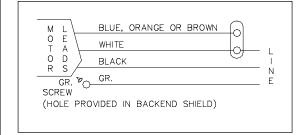
For any permanent split capacitor motor, which has four (4) leads is as follows: Brown leads to capacitor. Black-leads to Power Source.
