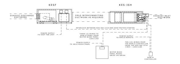
Remote wiring of KES Enviro units with Water Wash Hood and Panel Figure 8
