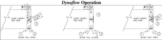
The internal blade (IB) is adjusted to direct fresh air between the Kitchen Ambient (3) Region, the Appliance (1) Region, and Chef(2) Region. The Comfort Tuning Blade (CTB) is adjusted to direct fresh air between the Appliance (1) Region and the Chef(2) Region. The complete kitchen ventilation system is always balanced. The IB and CTB are adjustable
