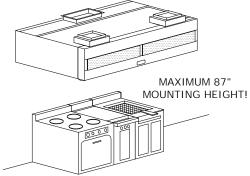
then discharges into the *Dynaflow* plenum. Within the plenum the fresh air is routed to three (3) regions within the boundaries of the appliances.
