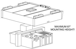
kitchen lineup. The MJ Perimeter Defense hood can be finetuned to provide excellent smoke capture with maximum grease extraction.
