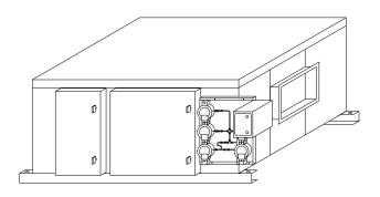
ISH. The link temperature is 165F and is accessible through the prefilters/Bag filter access door.
